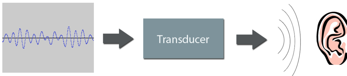
Figure 3: Electrical signal to sound pressure transduction
